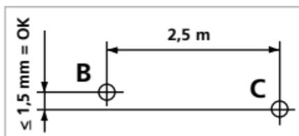
! Regularly check the calibration before use, after transport and after extended periods of storage.
