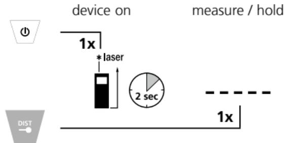
! After switching on, the device starts with continuous measurement.
