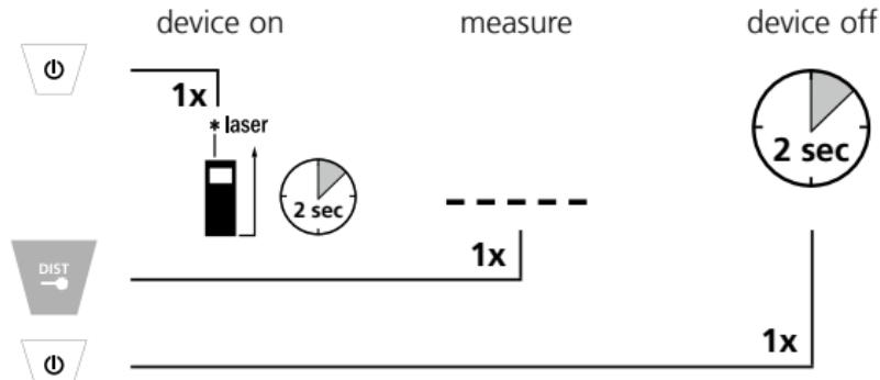
! After switching on, the device starts with continuous measurement.
