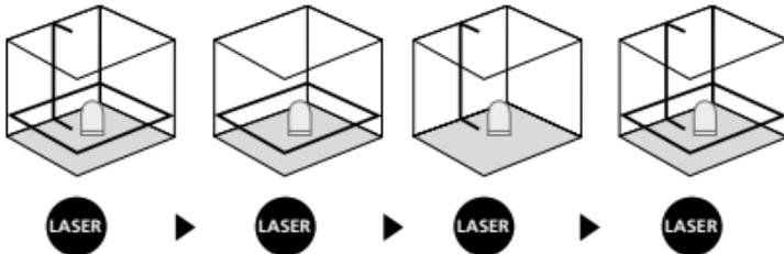
**!** The transport restraint must be released for horizontal and vertical levelling. The laser lines flash and the LED lights red as soon as the device is outside the automatic levelling range of 4°. Position the device such that it is within the levelling range. The LED switches back to green and the laser lines stop flashing (steady light).
