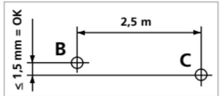
approx. 2.5 m to the right and mark point C. Check whether the horizontal line from point C is level with point B to within  $\pm 2$  mm. Repeat the process by turning the laser to the left.
