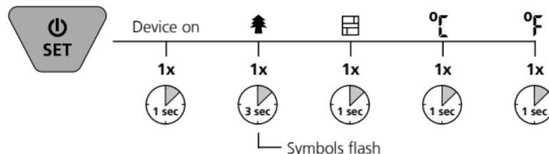
! The device starts with the measuring mode last selected. To select the mode, press and hold the Set button for 3 seconds or briefly wait until the symbol stops flashing.
