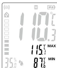
MAX/MIN mode refers to the infrared temperature and shows the maximum and minimum infrared temperature. The MAX/MIN values are determined while measuring when the trigger (8) is pressed. The value is deleted and calculated again at the start of a new measurement or by pressing the trigger (8).
