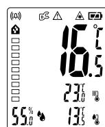
Ambient temperature/surface temperature differential:  $\geq 6.5^\circ\text{C}$  thermal bridge, Blue display and the “ $\Delta$ ” symbol flashes!
