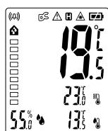
Ambient temperature/surface temperature differential:  $\geq 3.5^\circ\text{C}$  possible thermal bridge, the “ $\Delta$ ” flashes, check area again
