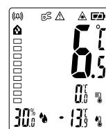
Ambient temperature/surface temperature differential:  $\geq -6.5^\circ\text{C}$  thermal bridge, Red display and the “ $\Delta$ ” symbol flashes
