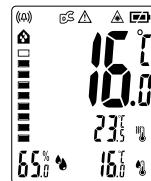
Risk of condensation moisture „
