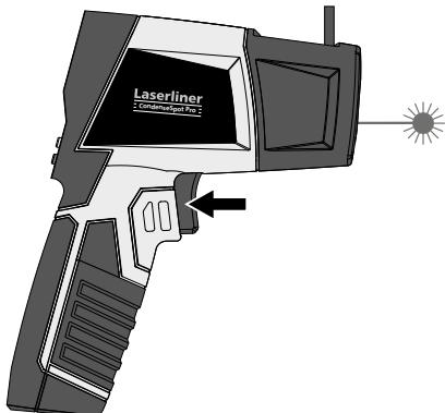
Release the button as soon as the target laser pinpoints the measurement location. The measured value is held (Hold).
