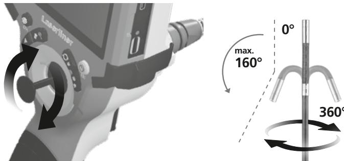
The factory setting for the maximum angular position of the 3D camera head is 160° in new condition, with a tolerance of  $\pm 5^\circ$ . To achieve this, the camera probe must be totally straight, meaning without any unnecessary curves or bends. The maximum angular position may be reduced by normal mechanical wear over the lifetime of the product.
