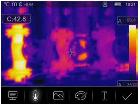
Pressing the trigger freezes the image and the save menu appears. The shot can be edited in the save menu before it is saved. There is an option for adding text comments. Pressing the text notes symbol opens an editor with a keyboard. Use the tick symbol to close the editor after entering the text.
