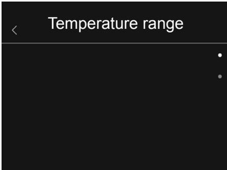
The default setting for the temperature range can be selected in this menu. Choose between two ranges: -20 - +150 °C (optimum for indoor and outdoor thermal imaging of buildings) 0 - +650 °C (optimum for industrial applications)
