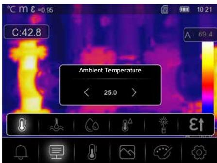
Influences measurements taken with the thermal imaging camera are affected by the ambient temperature. This parameter compensates the influence of the ambient temperature on the measurement. This can be set between 0 °C and 50 °C.
