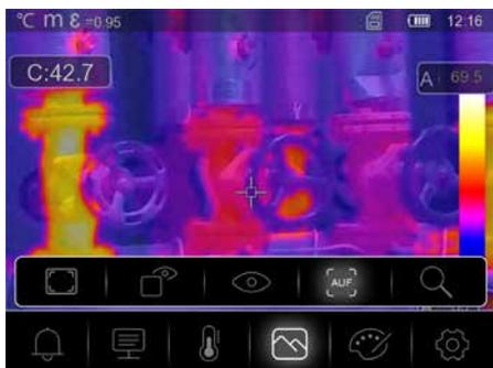
In **Auto Fusion** mode, the digital image and infrared image are overlaid. This allows the location of the relevant infrared areas to be quickly and precisely identified. The temperature in the central area is compared to the digital image. The mix ratio between the infrared image and the digital image can be adjusted manually. The detail of the overlaid area occupies approximately half the display area and is placed centrally but can be moved to a specific position using the touchscreen.
