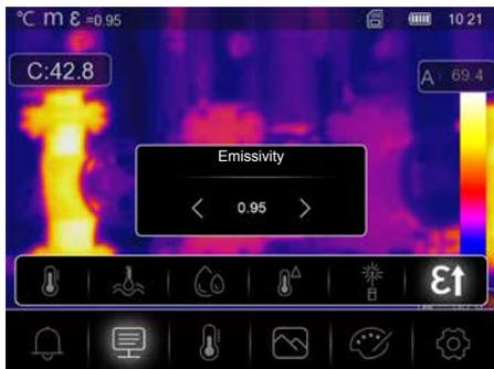
The level of infrared emissions given off by everything depends on the specific material and surface. This factor is determined by the emissivity coefficient (0.10 ... 1.0). For accurate measurements, it is absolutely essential that the emissivity coefficient is set first. The emissivity coefficient can either be custom set or selected based on the predefined emissivity coefficients from the material list.
