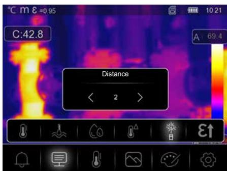
Air contains many different substances which can absorb infrared rays. The infrared radiation from the inspected object therefore decreases as the distance increases. At distances greater than 10 metres, the atmospheric influences of the air must always be taken into account. The distance can be set between 0 and 2,000 m.
