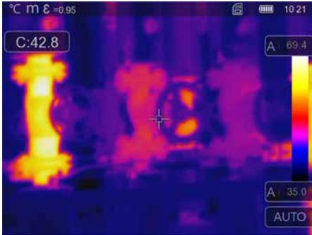
**A** In Automatic mode, the measured temperature range of the infrared image and the resultant distribution of the colour spectrum are permanently set. The colour spectrum of the measured infrared image is determined by the temperature range and colour scale. The colour distribution of the infrared image is automatically and dynamically adjusted in the bargraph based on the measured min./max. values.
