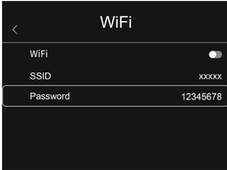
A connection to the device can be established via WiFi. The default SSID is 'TCHS' or 'TCHS Pro' and the default password is '12345678'. Data on the camera can be accessed using the Laserliner HighSense app once a connection is made.
