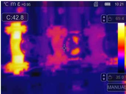
**🔒** In manual settings mode, the temperature range is no longer set automatically based on the measured min./max. values but rather determined on the basis of manual values.
