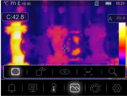
In **IR Thermal** mode, only the infrared image is shown.
