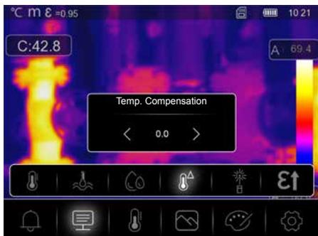
The temperature compensation can be set between -5.0 °C and +5.0 °C.
