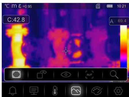
There are five different image modes for display: IR Thermal, MIX Image, Visible image, Auto Fusion, Zoom.
