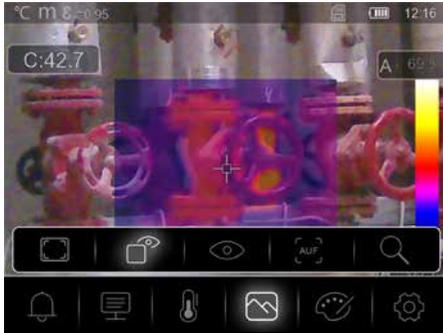
In **MIX Image** mode, a detail from the infrared image is displayed in the digital image.
