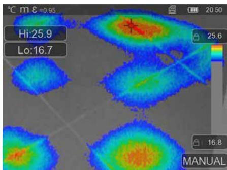
**FloorHeating-Control** provides visualisation of cable routing, thermal distribution and possible air inclusions. It allows you to check that an existing or recently installed underfloor heating system is heating up evenly. The thermal imaging camera provides information on the floor surface temperature which is also an important indicator of the heating system's efficiency.
