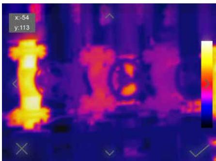
The digital image and infrared image can be aligned to each other using the arrow keys.
