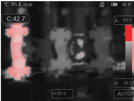
Areas with a temperature that exceeds the threshold set for the upper temperature are shown in red.
