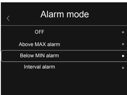
The upper and low alarm levels can be activated in the Alarm Mode menu.
