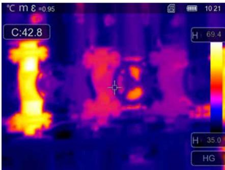
**H** In Histogram mode, the colour distribution of the infrared image is adjusted in the same way as in Automatic mode. In addition, a statistical analysis of the temperature distribution in the infrared image (histogram) stabilises the min.max. values. If the temperatures vary significantly, this stabilises the view from one image to the next, e.g. when measuring moving objects
