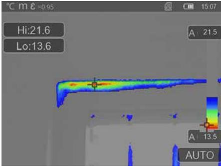
**LeakageControl** identifies cold spots where moisture can condense and damage from leaks may occur. These are the points in a building which transfer heat from inside to outside in a short space of time and thus cool more quickly than the surrounding areas. Early identification and treatment of these areas prevent subsequent mildew.
