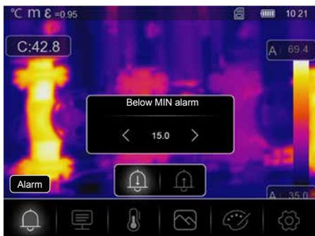
The alarm threshold values above and below the specified temperature levels can be set in this menu. Instructions for activating the alarm are provided in Section 14.3.
