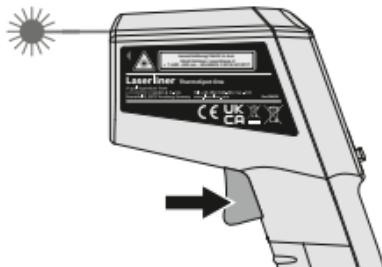
Release the button as soon as the target laser pinpoints the measurement location. The measured value is held.
