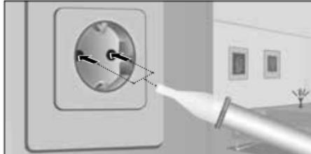
Position the detector tip in the area to be tested (e.g. cable, socket, etc.).
