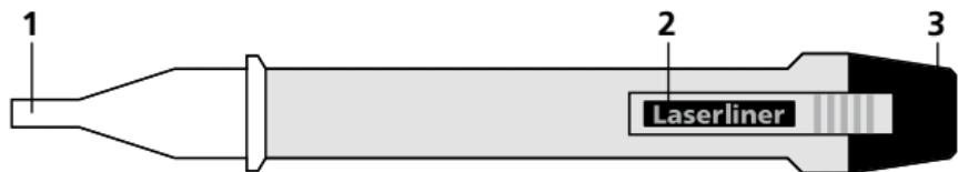
1 Detector tip      2 Pocket clip      3 Battery compartment
