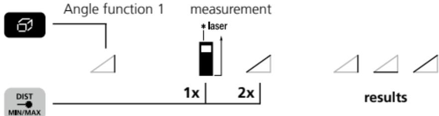
The measurement results are determined automatically by the 360° inclination sensor.
