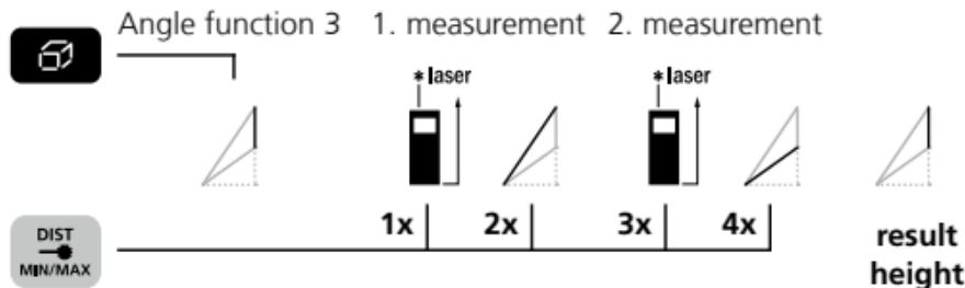
The measurement result is determined by the 360° inclination sensor.
