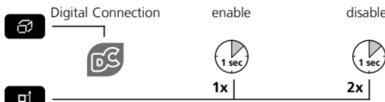
When enabled the Digital Connection symbol appears on the display (e). When the function is active, a mobile device can connect by means of an app to the measuring device.
