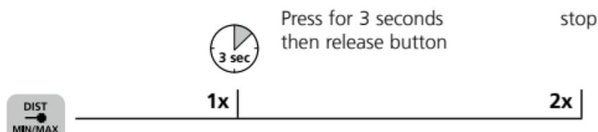
The LC display shows the max value, the min value and the current value.
