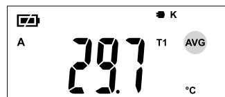
**A** Press button A to show the MAX, MIN, AVG values of thermocouple T1 as well as the difference T2-T1.
