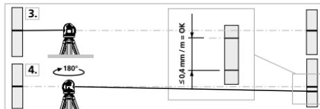
! When A2 and A3 are more than 0.4 mm / m apart, an adjustment is necessary.
