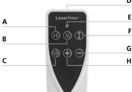
**A** Horizontal laser lines**B** Vertical laser lines**C** auto/man function /
