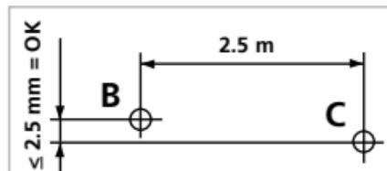
approx. 2.5 m to the right and mark point C. Check whether the horizontal line from point C is level with point B to within  $\pm 2,5$  mm. Repeat the process by turning the laser to the left.
