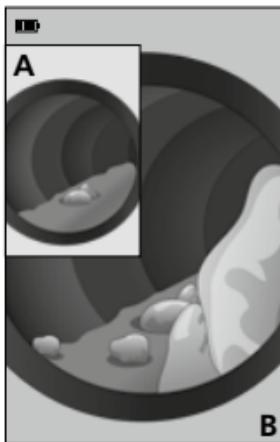
4. Selected reference image (A) appears on the display, the live view is running in the background (B) for comparison.
