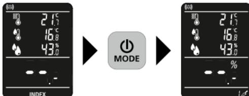
The device features 2 modes for measuring moisture, depending on the material in question. Press the 'MODE' button to change between the central, material-independent INDEX mode and the additional Building Material mode.
