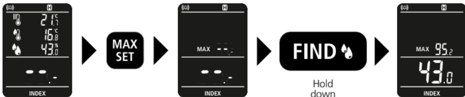
The device can only retain a MAX value as part of a measuring process. The MAX value is displayed after the measuring process. The MAX value and the current value are displayed by holding down the 'FIND' button during a new measurement.
