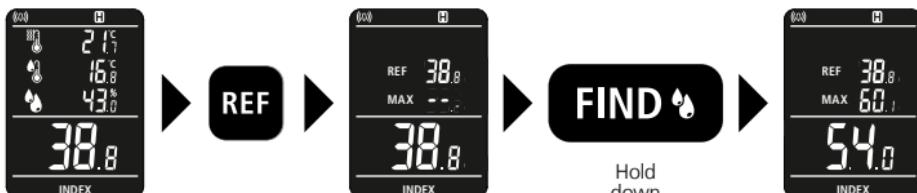
The Reference function allows you to gain an overview of the moisture distribution in the wall. Find a dry point on the item to be measured and determine the moisture content as described in section 6 "Measuring process". Fix the measured value as a reference value by pressing the 'REF' button. Then complete a moisture measurement elsewhere. This gives you an overview from the reference value, maximum measured value and current measured value.
