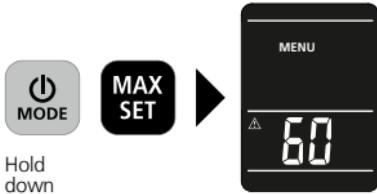
Holding down the ON/OFF button and the MAX button at the same time takes you to the menu. The dry limit value, alarm and automatic power off can be set from here.
