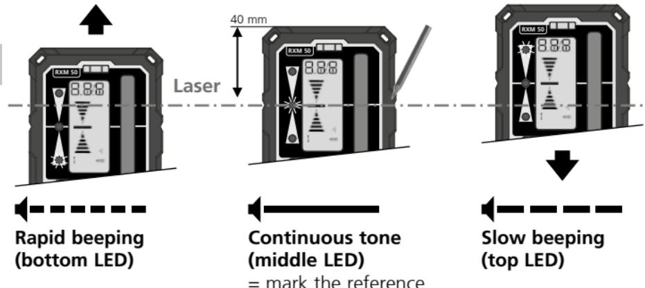
**!** The light intensity of the laser lines is greatest at the centre and diminishes toward the ends. This can reduce the maximum reception range of the laser receiver.
