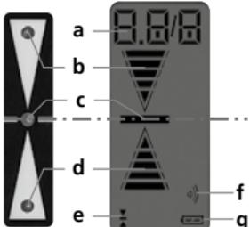
**a** Numerical deviation from the laser level**b** Hand receiver above laser level**c** Precisely on laser level**d** Hand receiver below laser level**e** Accuracy (3-stage)**f** Sound ON / OFF**g** Low battery indicator
